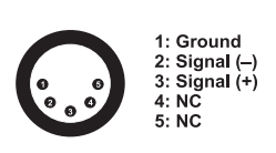
DMX-input XLR mounting-plug:
