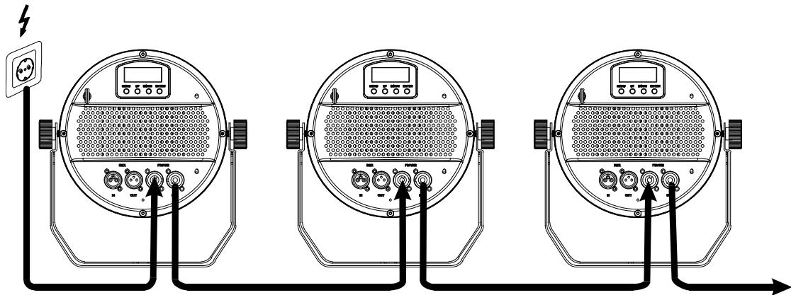
The device uses an auto-range power supply that accepts input voltages between 100 und 240 volts.
