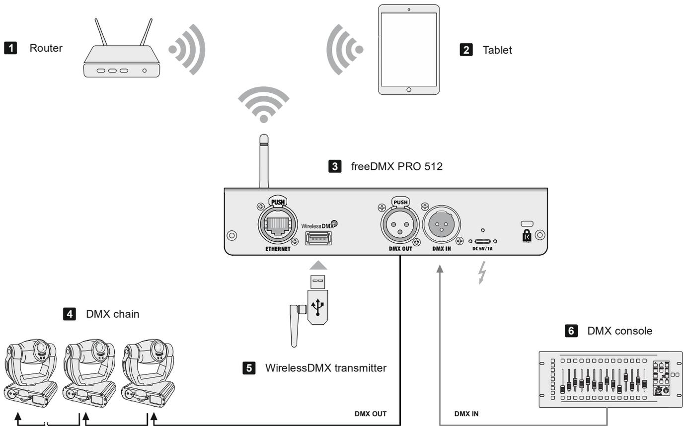
Your tablet can be connected either directly or via an existing network. The XLR socket or a WirelessDMX transmitter can be used for DMX output. As an alternative to the Wi-Fi signal, connect a DMX console for DMX input. Use this input option, for example, for a backup system or merger operation, where you set the basic mood with the house console and combine it with motion effects from the tablet. Below are various examples of standard applications and the necessary configuration steps.
