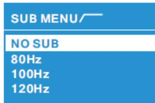
The SUB menu is used to select a high-pass frequency for use with a subwoofer. By filtering the low frequencies, the efficiency between the full-range speaker and the subwoofer can be balanced. Available options for this selection are: 80Hz, 100Hz, 120Hz. The default is “No Sub”.
