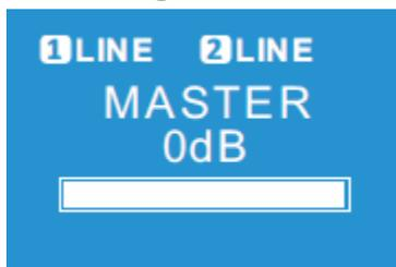
After switching on, the display indicates "Loading" while the unit starts up. After a few seconds, the main screen is displayed and you can adjust the overall volume with the MASTER VOL knob (2) in the range of -60 dB to 0 dB. In the upper line of the main screen, the status of both mono channels is displayed.
