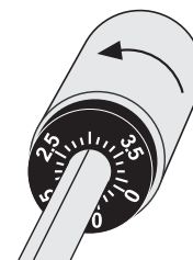
Fig. 6: Stylus pressure adjustment
